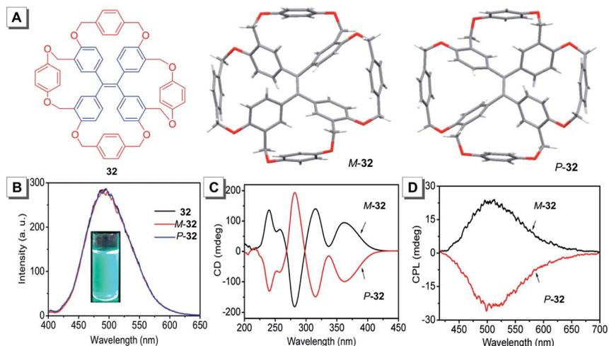
Fig. 16 (A) Molecular structure of **32** and its crystal structures. (B) PL spectra of racemic-**32**, *M*-**32** and *P*-**32** in THF ( $[32] = 5.0 \times 10^{-5}$  M). (C) CD spectra and (D) CPL spectra of *M*-**32** and *P*-**32** in THF ( $[32] = 1.0 \times 10^{-3}$  M). Adapted from ref. 79 with permission. Copyright 2016 American Chemical Society.
