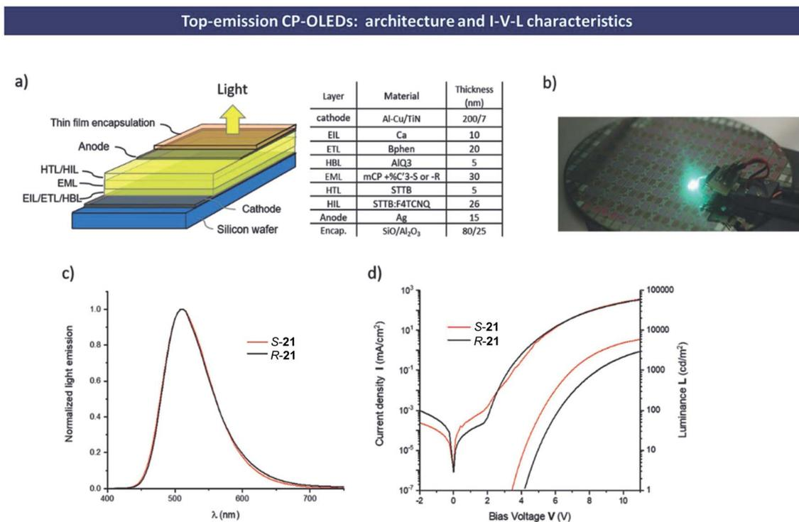
Fig. 21 (a) Device structure of a top-emission CP-OLED built from a typical thin film stacked with *R*-21 and *S*-21 chiral dopants. (b) The test of an individual CPOLED in 8 inch wafer level-processed CP-OLEDs. (c) Light emission spectrum of CP-OLEDs integrating either *S*-21 or *R*-21 chiral dopants; (d) corresponding *I*-*V*-*L* characteristics. Adapted from ref. 69 with permission. Copyright 2020 Wiley-VCH.
