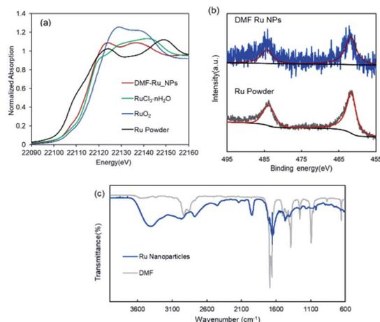
Fig. 2 (a) Ru K-edge XANES spectra of DMF-stabilized Ru NPs (red), RuO<sub>2</sub>, and Ru powder; (b) Ru 3p XPS spectra of DMF-stabilized Ru NPs (blue) and Ru powder (gray); and (c) FT-IR spectra of DMF-stabilized Ru NPs (blue) and DMF (gray).
