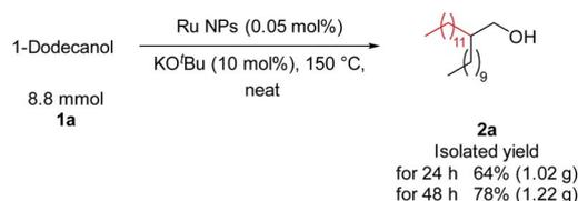
Fig. 5 1 g scale synthesis of **2a**.
