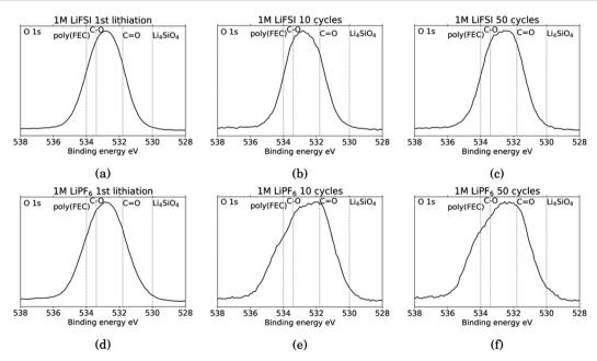
Fig. 6 O 1s spectra for Si electrodes cycled to 1st lithiation, cycle 10 and cycle 50 in LiFSI (a-c) respectively, and in LiFF<sub>6</sub> (d-f) respectively.
