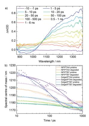
Fig. 4 (a) TA spectrum for degraded nanoparticle  $ZnO/AgBiS_2-TMAI/PTB7$  device following a 700 nm pump excitation. (b) Centre of mass of PIA signal as a function of time for each device configuration.
