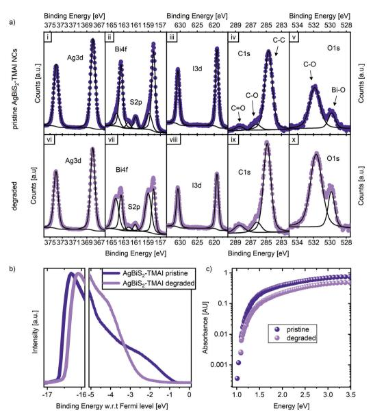
Fig. 5 The degradation of AqBiS<sub>2</sub>-TMAI NCs. (a) XPS data of a pristine film in the top row, bottom row presents the state after 24 h of dry air and sunlight exposure. The scale is arbitrary but the same for each orbital. (b) UPS data for a pristine and 17 h degraded AgBiS2-TMAI film on ITO. (c) PDS measurement of the absorption of a pristine and 24 h degraded film.
