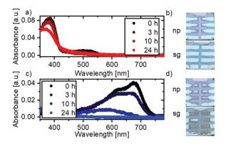
Fig. 6 Dry air and sunlight degradation of the HTL. (a) Absorption changes of a PTAA:C<sub>60</sub>F<sub>48</sub> film. (b) Picture of the electrode of a device using PTAA: $C_{60}F_{48}$  after 42 h of degradation with either ZnO nano-particle or sol-gel as ETL. (c) Absorption changes in PTB7. (d) Pictures of solar cell electrodes employing PTB7 as HTL and either nano-particle or sol-gel ZnO as ETL.
