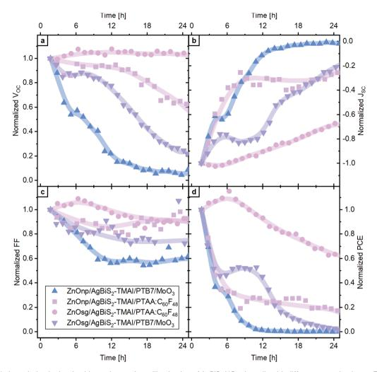
Fig. 2 Photovoltaic evolution in dry air with continuous 1 sun illumination of AgBiS<sub>2</sub> NC solar cells with different extraction layers. The photovoltaic parameters, (a) V<sub>OC</sub>, (b) J<sub>SC</sub>, (c) FF and (d) PCE, were averaged from several devices and normalized to their initial value. A guide for the eye in form of a line is added.
