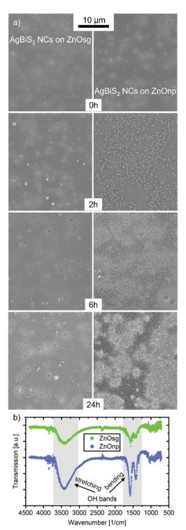
Fig. 7 (a) SEM pictures of a  $AgBiS_2$ -TMAI NC film on a ITO/ZnOsg (left column) or np (right column) layer during degradation in dry air and sunlight for different time steps. (b) FTIR measurements of a pristine ZnOsg and np film. The OH vibration bands are indicated and the data is offset to each other for better visibility.
