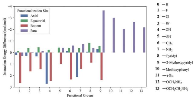
**Fig. 14** Calculated CO<sub>2</sub> interaction energies of functionalized calixarenes. All energies are given as a difference from the interaction energy of the unfunctionalized calixarenes ( $-6.82 \text{ kcal mol}^{-1}$ ). Reproduced with permission from ref. 166.
