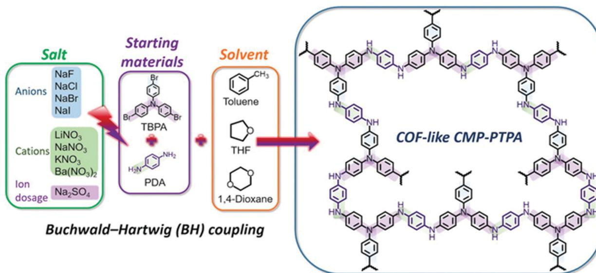
Fig. 11 Synthesis of salt-tunable CMP-PTPA by Buchwald–Hartwig (BH) cross-coupling. Reproduced with permission from ref. 146.
