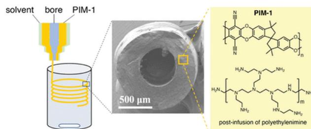
Fig. 12 Shaping PIM-1 into hollow fiber sorbents and polyethyleneimine impregnation in PIM-1. Reproduced with permission from ref. 158.
