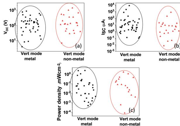
**Fig. 7** Comparison of the responses summarized in Tables 1 and 2 for the vertical mode of operation for metal-based devices (in black) and non-metal-based devices (in red) for  $V_{OC}$  (a),  $I_{SC}$  (b), and power output (c).
