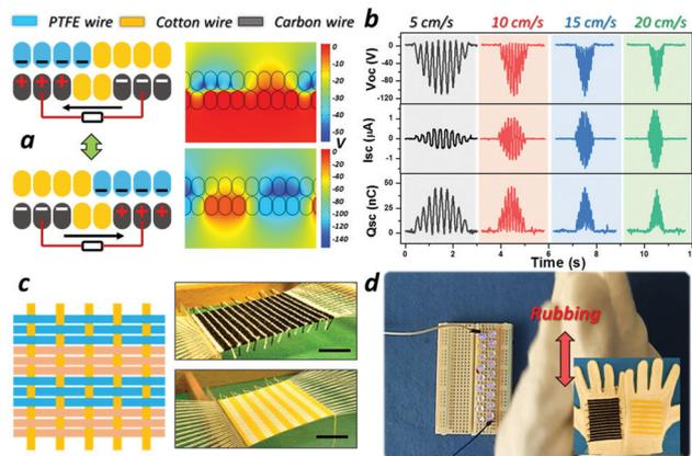
Fig. 6 (a) Scheme of the free-standing mode PTFE grating textile and interdigital carbon textile electrode for horizontal motion, (b) measurements of  $V_{oc}$ ,  $I_{sc}$ , and  $Q_{sc}$  under operation, (c and d) photographs of the electrode and sliding textile under operation with commercial blue LEDs. Reprinted from ref. 86. Copyright (2018), with permission from Elsevier.
