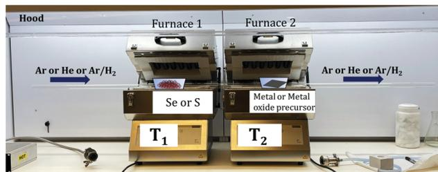
Fig. 6 Furnace-based ambient-pressure chemical vapor deposition (AP-CVD) setup in the Nessim Lab. This system is composed of two furnaces in series. Digital mass-flow controllers (MFCs) for many gases, including Ar, forming gas,  $H_2$ ,  $C_2H_4$ ,  $N_2$ , etc., control gas flow. In the first furnace, we sublime the chalcogen (S or Se) powder, while the reaction with the metal foil occurs in the second furnace. The two temperatures,  $T_1$  and  $T_2$ , can be independently controlled.
