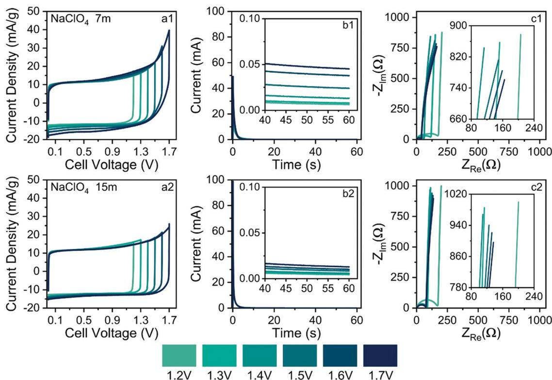
**Fig. 10** Electrochemical findings obtained using the CV (a), SSC (b), and EIS (c) techniques. Conditions: (a–c)(1)  $7.0\text{ mol kg}^{-1}$   $\text{NaClO}_4$ , and (a–c)(2)  $15.0\text{ mol kg}^{-1}$   $\text{NaClO}_4$ .  $\nu = 1\text{ mV s}^{-1}$ . Electrode: MWCNTs.
