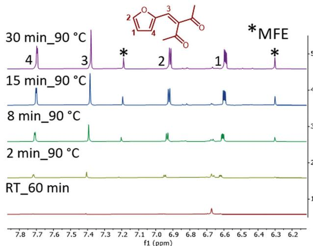
**Fig. 1** <sup>1</sup>H NMR spectra of the organic phase in xylose\_acac\_ZrCl<sub>4</sub>\_NaCl reaction at room temperature (RT) for 60 min; at 90 °C for 2 min, 8 min, 15 min and 30 min, respectively. Reaction conditions: 2 mmol xylose, 20 mol% ZrCl<sub>4</sub>, 2 mL D<sub>2</sub>O (with 10 mmol NaCl), 2 mL acac were added into a vial and reacted in an oil bath at 90 °C for a certain number of minutes.
