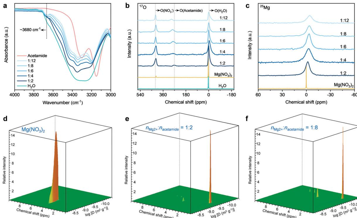
Fig. 2 Spectroscopic characterizations of the electrolytes. (a) FT-IR, (b) liquid-state  $^{17}\text{O}$  NMR, and (c) liquid-state  $^{25}\text{Mg}$  NMR spectra. PFT-NMR contour spectra of (d) 1 M  $\text{Mg}(\text{NO}_3)_2$ , (e) the electrolyte with  $n_{\text{Mg}^{2+}} : n_{\text{acetamide}} = 1 : 2$ , and (f) the electrolyte with  $n_{\text{Mg}^{2+}} : n_{\text{acetamide}} = 1 : 8$ .
