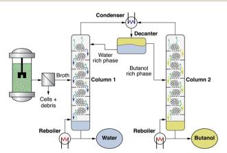
Fig. 9 Illustration of heteroazeotropic distillation for the separation of butnanols from fermentation broth. A detailed set of operation parameters for these columns can be found in Luyben, 2008.<sup>210</sup>
