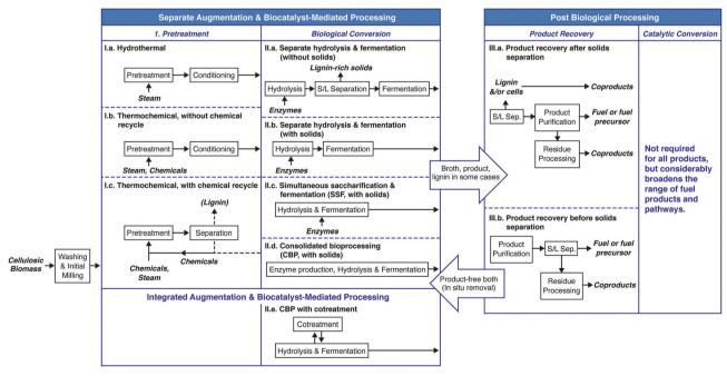
Fig. 4 Processing landscape for conversion of lignocellulose to fuels. See text for explanation
