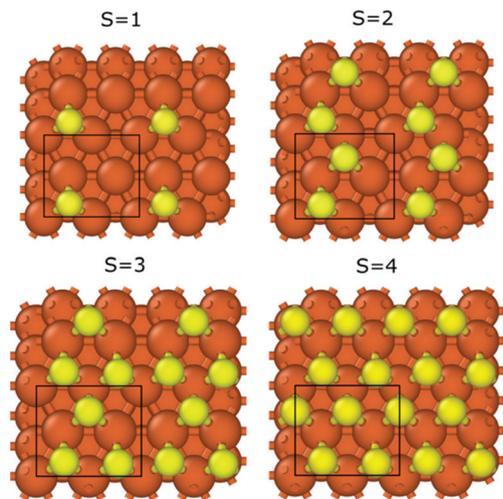
**Fig. 3** Top view of the iron surface configurations with different sulfur coverages. Black rectangles represent the applied cells in the computations, while  $S$  corresponds to the number of sulfur atoms in the cell.
