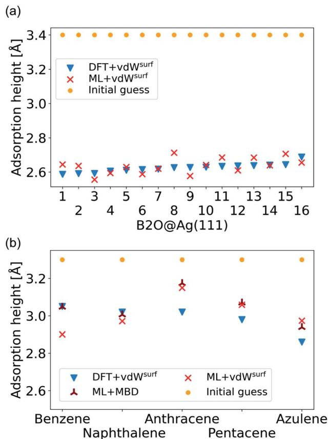
Fig. 6 (a) Adsorption heights of B2O molecules on Ag(111). (b) Adsorption heights of benzene,<sup>82</sup> naphthalene,<sup>83</sup> anthracene,<sup>84</sup> pentacene,<sup>85</sup> and azulene,<sup>83</sup> computed with ML+vdW<sup>surf</sup> and compared to DFT+vdW<sup>surf</sup>. The same adsorption sites as mentioned in the cited references (Table 1) are used.
