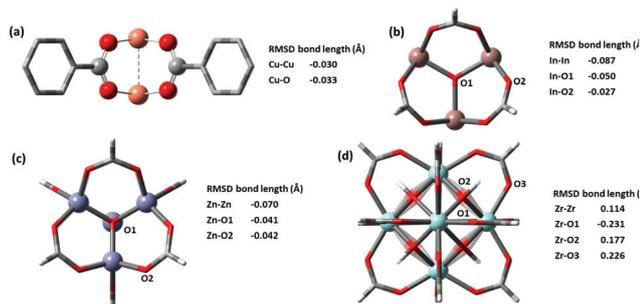
Fig. 4 (a) Cu-based Paddlewheel  $M_2O$  of refcode FIQCEN<sup>86</sup> (b) In-based Trimeric Oxo-centred  $M_3O$  refcode FIGIM<sup>87</sup> (c) Zn-based octahedron  $M_4O$  of refcode EDUSIF<sup>88</sup> (d) Zr-based cubo-hedral  $M_6O$  of refcode RUBTAK03.<sup>89</sup> Crystal structure is represented by opaque and optimized structures are shown partly transparent.
