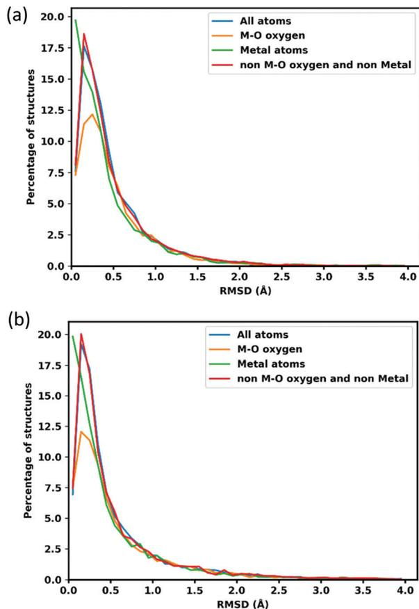
Fig. 2 RMSD of GFN-xTB optimized atom positions with respect to the CoRE structures. (a) Shows optimization allowing only atom position movement. (b) Shows optimization where both the lattice and atomic positions were allowed to relax.
