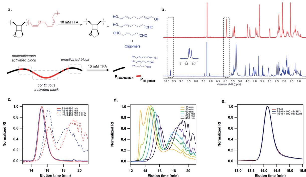
Fig. 3 (a) Acid degradation of mechanically activated polymer. (b)  $^1\text{H}$  NMR spectra of mechanically activated poly(1) before (top, red trace) and after (bottom, blue trace) 10 mM TFA treatment. (c) GPC traces of hydrogenated poly(1) showing resistance to acidic and basic hydrolysis. (d) GPC traces of activated P1-H at different times after 10 mM TFA treatment. (e) Comparison of GPC traces of P1-H and P2-H after 480 min of sonication and 10 mM TFA treatment.
