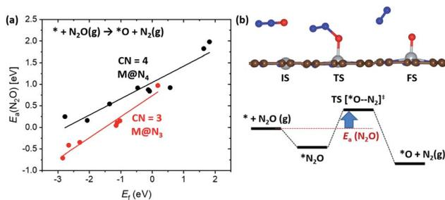
Fig. 5 (a) Shifted linear scaling relationships between  $E_f$  and  $E_a(N_2O)$  determined by CN. Black and red data points represent  $M@N_4$  and  $M@N_3$ , respectively. (b) The optimized geometries of the IS, TS and FS for  $^*O$  formation when using  $N_2O$  and associated energy diagram for  $E_a(N_2O)$ .  $E_a(N_2O) < 0$  eV indicates that  $^*O$  formation proceeds *via* exothermic  $N_2O$  adsorption and low activation energy.
