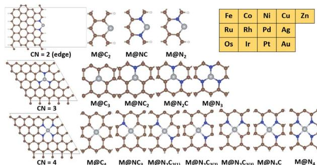
Fig. 2 Calculation models for  $M@N_xC_y$  catalysts. Grey, brown, blue and white balls represent transition metal, carbon, nitrogen and hydrogen atoms, respectively. The 13 late transition metals considered in this study are shown as a table.
