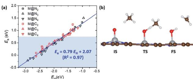
Fig. 4 (a) Linear scaling relationship between  $E_H$  and  $E_a$ . The area shaded in blue is  $E_a < 0.75$  eV. (b) The optimized geometries for the initial state (IS), transition state (TS) and final state (FS) in methane activation.
