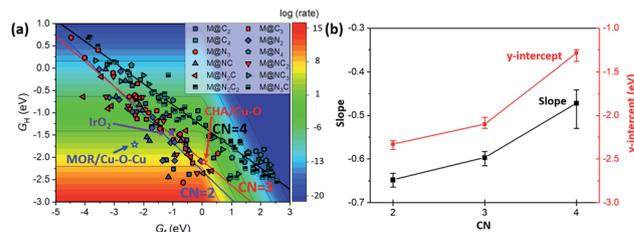
Fig. 3 (a) 2D-volcano plot for methane activation at 150 °C as a function of  $G_f$  and  $G_H$ . Blue, red and black lines represent linear scaling lines of CN = 2, 3 and 4, respectively. (b) Changes in the slope and  $y$ -intercept of the linear scaling line with CN. Each data point represents an average value, while the error bar represents the range of slopes (or  $y$ -intercepts) at each CN.
