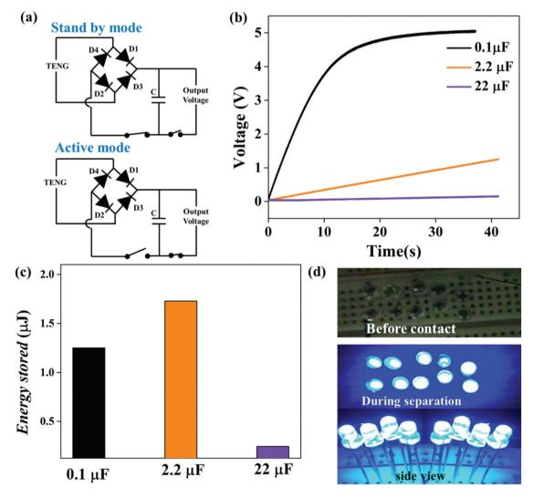
Fig. 6 Schematic diagram of the charging circuit (a) and (b) the DL<sub>2</sub> device deployed to generate the voltage stored in different capacitors, (c) the amount of energy stored in various capacitors, and (d) the digital image of ten LEDs lighten up by charged capacitor.
