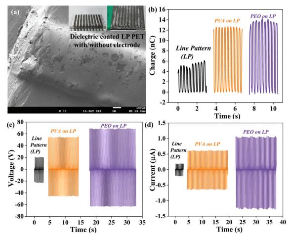
Fig. 3 (a) Photographic image of the dielectric coated with and without electrode LP PET (b) transfer charges of single and double-layered TENG (c) and (d)  $V_{\rm oc}$  and  $I_{\rm sc}$  measurement of DL<sub>1</sub> and DL<sub>2</sub> TENG devices with the fixed operational parameters i.e., frequency of 5 Hz, CS distance 4 mm, and a force of 50 N.
