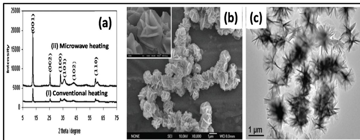
Fig. 8 (a) XRD pattern of  $\alpha$ -Ni(OH)<sub>2</sub> synthesized by (i) conventional heating method and (ii) MW heating method.<sup>178</sup> (b) SEM image of  $\alpha$ -Ni(OH)<sub>2</sub> and (c) TEM image of  $\alpha$ -Ni(OH)<sub>2</sub>.<sup>179</sup> Reprinted (adapted) with permission from ref. 178 and 179, copyright (2008 and 2010), the American Chemical Society.
