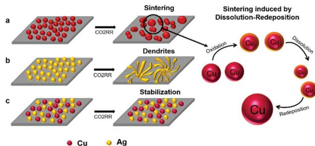
**Fig. 8** Schematic illustration of the structural evolution of (a) Cu, (b) Ag and (c) Cu–Ag NP electrodes under electrochemical CO<sub>2</sub>RR conditions (−0.8 V vs. RHE), and the observed stabilization effect in binary Cu–Ag nanoparticle electrodes.
