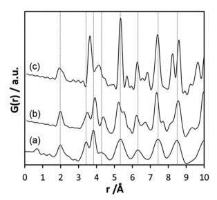
Fig. 10 (a) Experimental PDF obtained at 700 °C during heating of  $d-Ta_xO_v$ , calculated PDFs based on the structures of (b) L-Ta<sub>2</sub>O<sub>5</sub><sup>13</sup> and (c)  $\beta$ -Ta<sub>2</sub>O<sub>5</sub>. <sup>14</sup>
