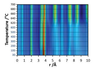
Fig. 7 False colour heat map of PDFs obtained from in situ heating experiments carried out under synthetic air on d-Ta<sub>x</sub>O<sub>v</sub> powder sample. Data for PDF were collected every 50 °C between room temperature and 600 °C and every 10 °C between 600 and 700 °C (red colour indicates high intensities, blue colour low intensity).
