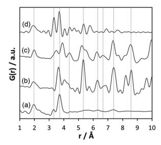
Fig. 5 (a) Experimental PDF obtained from h-Ta<sub>x</sub>O<sub>v</sub>H<sub>z</sub>, (b) simulated PDF of  $\beta$ -Ta<sub>2</sub>O<sub>5</sub>, <sup>14</sup> (c) simulated PDF of L-Ta<sub>2</sub>O<sub>5</sub> structure, <sup>13</sup> (d) simulated PDF based on Abrahams' structure of Ta<sub>8</sub>O<sub>10</sub>(OEt)<sub>20</sub>.50
