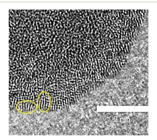
Fig. 6 High-resolution TEM image of d-Ta<sub>x</sub>O<sub>y</sub>. Small units showing a certain regularity are encircled.
