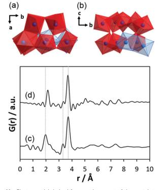
Fig. 11 Cluster model derived from cutting a part of the crystal structure of L-Ta<sub>2</sub>O<sub>5</sub> followed by a simple geometric optimisation: (a) top view and (b) side view. (c) Experimental PDF of h-Ta<sub>x</sub>O<sub>v</sub>H<sub>z</sub> is given in comparison to (d) the PDF calculated based on this structure.
