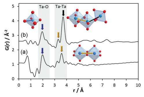
Fig. 3 Experimental PDFs of (a) Ta<sub>2</sub>(OEt)<sub>10</sub> and (b) h-Ta<sub>x</sub>O<sub>v</sub>H<sub>z</sub>. The main pair correlations are marked by arrows with the blue one representing individual Ta-O distances within an octahedron, the yellow one labels Ta-Ta distances between edge-sharing octahedra, and the black one highlights Ta-Ta distances between corner-sharing octahedra.
