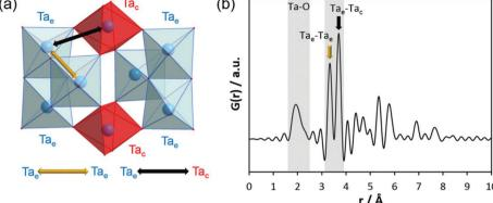
Fig. 4 (a) Model of connected trinuclear units  $[Ta_8(\mu_3-O)_2(\mu-O)_8(\mu-OE)_6(OE)_{14}]$ , based on crystal structure data published for tantalum ethoxide hydrolysed in alcohol by Abrahams et al. 50 and (b) simulated PDF of that structure.
