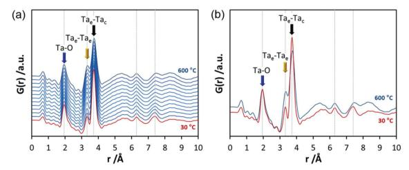
Fig. 8 (a) Experimental PDFs obtained during heating of d-Ta<sub>x</sub>O<sub>y</sub> from room temperature to 600 °C. (b) Comparison of the experimental PDFs obtained at 30 °C and in situ at 600 °C. The atom pairs corresponding to Ta-O distances within the octahedra, between edge-sharing octahedra, and between edge- and corner-sharing octahedra are marked with blue, yellow, and black arrows.
