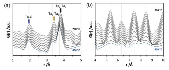
Fig. 9 Experimental PDFs obtained during heating of d-Ta<sub>x</sub>O<sub>y</sub> between 600 and 700 °C (a) displayed for the r-range between 1 and 5 Å, (b) in the r-range between 4 and 10 Å. The atom pairs corresponding to Ta-O distances within the octahedra, between edge-sharing octahedra and between edge- and corner-sharing octahedra are marked with blue, yellow and black arrows.
