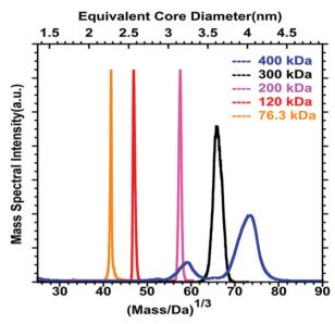
Fig. 2 MALDI-MS of 76.3 to 400 kDa nanoparticles synthesized using  $HSC_6H_{13}$  thiol. Mass spectrum data are plotted *versus* the cube root of mass to allow comparison with the core equivalent diameter (reprinted with permission Copyright© 2018 American Chemistry Society).<sup>45</sup>
