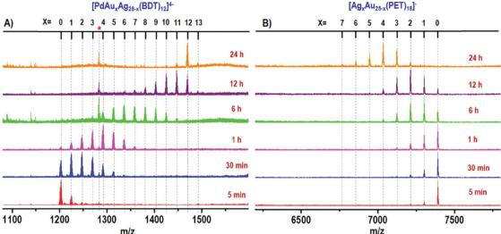
Fig. 4 Time-dependent ESI MS of intercluster reaction between PdAg<sub>28</sub> and Au<sub>25</sub> (1:5 ratio) where panel (A) shows the reaction at the PdAg<sub>28</sub> side and panel (B) presents the reaction at the Au<sub>25</sub> side. The red asterisk corresponds to thiolates produced during the reaction. The species observed are  $[PdAu_xAg_{28-x}(BDT)_{12}]^{4-}$  and  $[Ag_xAu_{25-x}(PET)_{18}]^-$ . (reprinted with permission Copyright © 2019 American Chemistry Society). (10)
