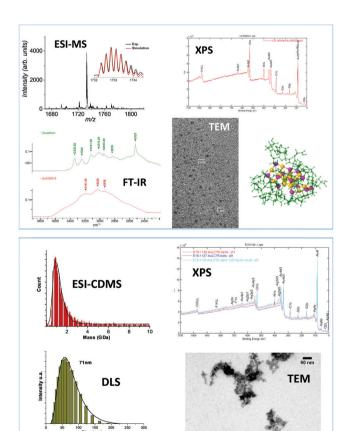
Fig. 12 Examples of characterization techniques in addition to mass spectrometry used for atomically precise  $Au_{15}SG_{13}$  nanoclusters (top panel) and Sub-100 nanometer silver doped gold-cysteine supramolecular assemblies (bottom panel). XPS: X-ray photoelectron spectroscopy, FT-IR: Fouriertransform IR spectroscopy, TEM: Transmission electron miscorscopy, DLS: dynamic light scattering.
