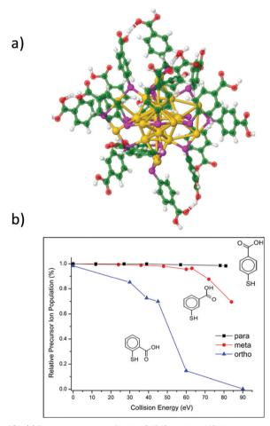
Fig. 10 (a) Proposed structure for  $Au_{25}(MBA)_{18}$  with p-MBA isomeric ligand. (b) CID breakdown curves for the 4-charge state of Au<sub>25</sub>(MBA)<sub>18</sub> for the three isomeric MBA ligands as a function of collision energy. (reprinted with permission Copyright © 2018 American Chemistry Society). 216
