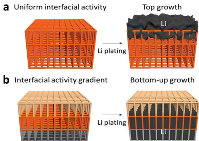
Fig. 10 Growth of lithium metal on the framework with (a) uniform interfacial activity and (b) interfacial activity gradient. The figures are reproduced from ref. 231.<sup>227</sup>
