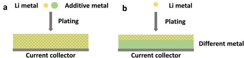
Fig. 8 Schematic illustration of lithium free anodes with lithium alloy formation. The alloy may form (a) by introducing an additive metal cation to the electrolyte, or (b) by alloying with a different metal substrate.
