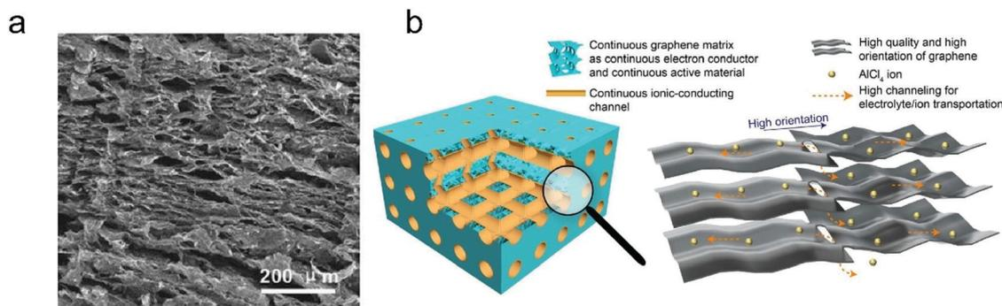
Fig. 13 (a) The SEM image of three-dimensional graphite foam. Reproduced from ref. 97 with permission from Wiley-VCH. (b) Illustration of tri-continuous and tri-high design for a desired graphene film. Reproduced from ref. 169 with permission from AAAS.
