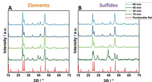
Fig. 1 Exemplified powder X-ray diffractograms of Pn-materials synthesized at different time scales (15–60 min) using  $8 \times 10$  mm  $ZrO_2$  balls and starting from an elemental reaction mixture (A,  $E_8$ -Y) or the respective metal sulfides (B,  $S_8$ -Y).
