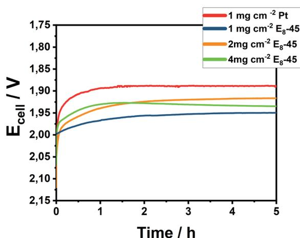
Fig. 6 Chronopotentiometry of Pt/C and E<sub>8</sub>-45/C at a catalytic loading of 1–4  $\text{mg cm}^{-2}$  at 80  $^{\circ}\text{C}$  for 5 h at an applied current of 1  $\text{A cm}^{-2}$ .
