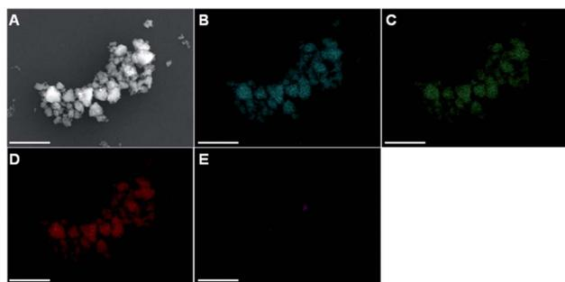
Fig. 2 (A) SEM image displaying the particles sizes and morphologies of E<sub>8</sub>-45. Further, EDX mappings reveal the presence of the elements (B) Fe (blue), (C) Ni (green), (D) sulfur (red) and (E) zirconium (violet). The scale bar is 2.5 μm.
