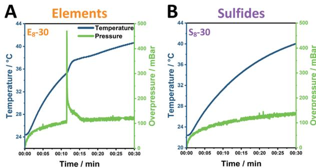
Fig. 4 Pressure- and temperature measurements during Pn synthesis employing (A) eight 10 mm ZrO<sub>2</sub> balls added to an elemental reaction mixture; (B) eight 10 mm ZrO<sub>2</sub> balls added to a sulfidic reaction mixture.
