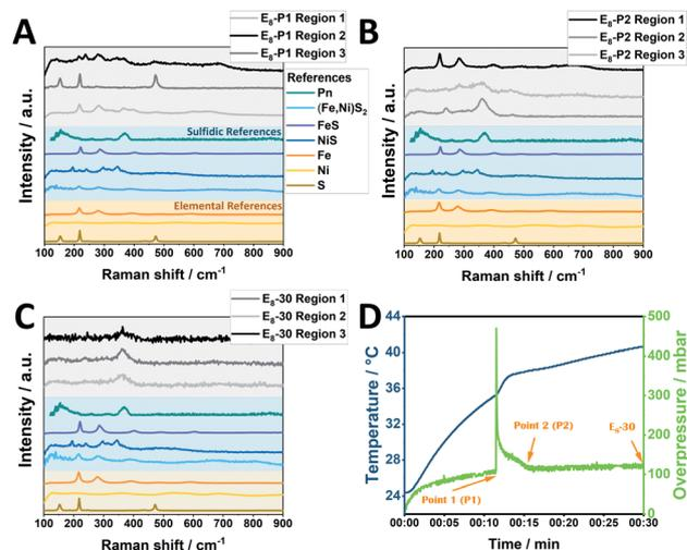
Fig. 5 Raman spectra of the obtained E<sub>8</sub>-Y samples at three different time points of the mechanochemical reaction: closely before the initiation of the MSR reaction (A), closely after (B) and after 30 min of milling (C). The respective points are also shown for clarity in (D).
