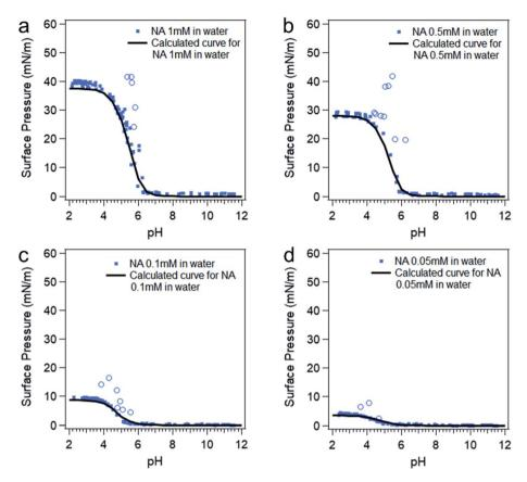
Fig. 2 Surface pressure *versus* pH curves at different nonanoic acid concentrations: experimental data (blue dots) and model calculated curves (black curves) using eqn (4), (5) and (7). The blue open circles represent the data due to the "soap effect" as discussed in detail in previous studies.<sup>20,56–59</sup>
