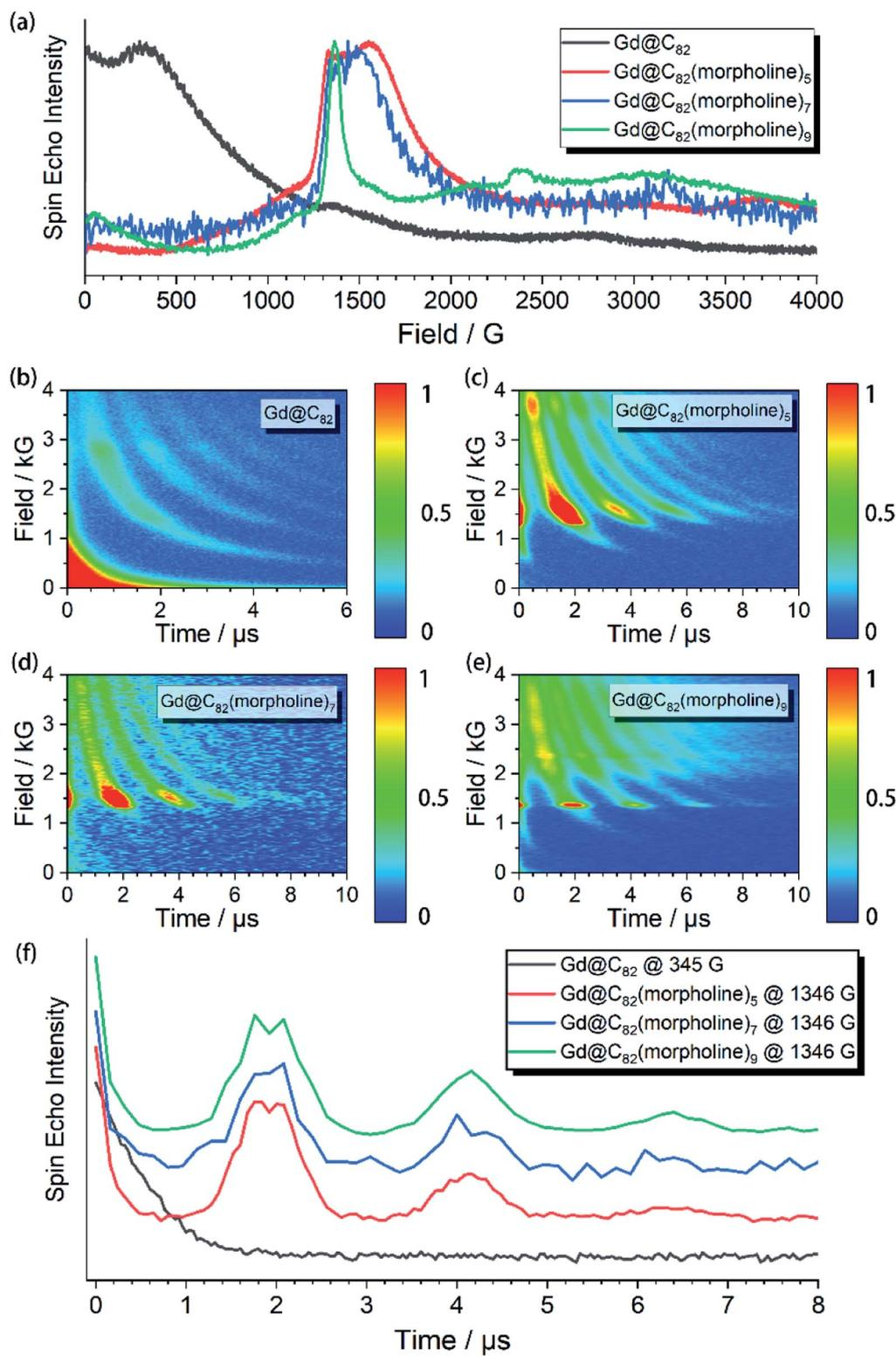
Fig. 2 (a) Echo-detected field swept spectra of  $\text{Gd@C}_{82}$  and the three derivatives  $\text{Gd-n}$  with normalized echo intensities; (b)–(e) the spin echo decay at different external applied magnetic fields ( $B_0$ ) of each compound; (f) decay of the Hahn-echo intensity as a function of delay time for  $\text{Gd@C}_{82}$  and the three derivatives  $\text{Gd-n}$  at specific  $B_0$ .
