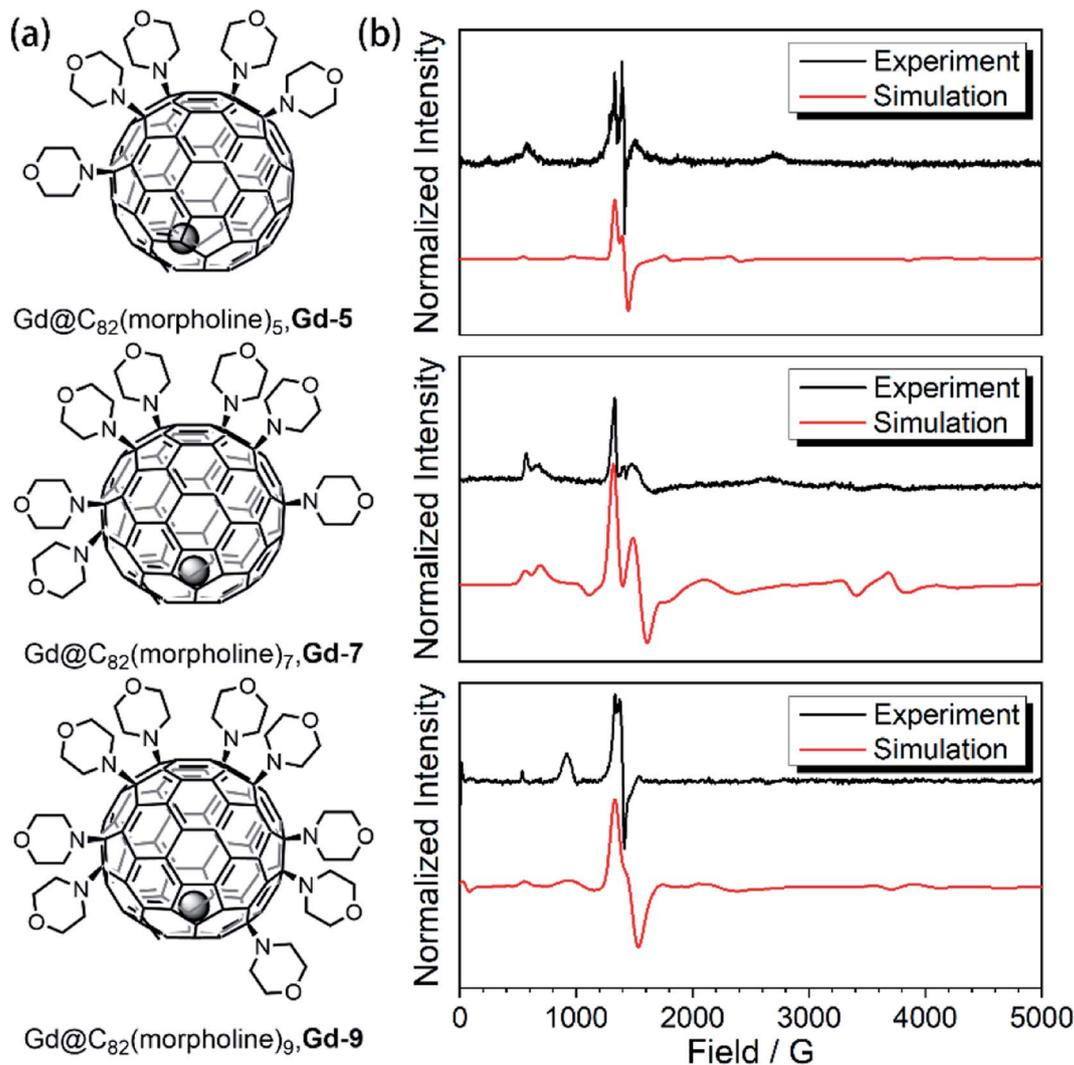
Fig. 1 (a) Aminated derivatives of Gd@C<sub>82</sub> with different numbers of morpholine groups. (b) The cw-EPR measurements for the Gd-*n* derivatives (black) and the best simulation results (red).
