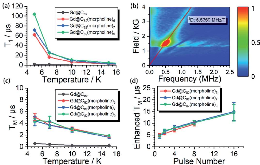
Fig. 3 (a) Spin–lattice relaxation time ( $T_1$ ) of  $\text{Gd}@C_{82}$  and the three derivatives  $\text{Gd-}n$ . (b) 2p-ESEEM spectrum at different external applied magnetic fields for  $\text{Gd-5}$ . The red line represents the simulation with the Larmor frequency of the  $^2\text{D}$  nuclear spin. (c) Spin–lattice relaxation time ( $T_1$ ) of  $\text{Gd}@C_{82}$  and the three derivatives  $\text{Gd-}n$ . (d) Dynamic decoupling results for the three derivatives  $\text{Gd-}n$ .
