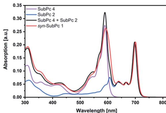
Fig. 3 Steady-state absorption spectra of *syn*-SubPc 1 ( $1.5 \times 10^{-6}$  M), dimer-SubPc 2 ( $1.5 \times 10^{-6}$  M) and monomer-SubPc 4 ( $3.0 \times 10^{-6}$  M) in toluene. The black spectrum relates to that of a 1 : 2 mixture of 2 and 4.
