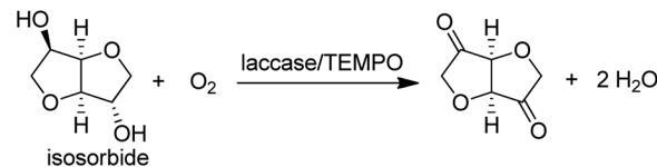
Scheme 12 Laccase/TEMPO catalysed oxidations of alcohols.
