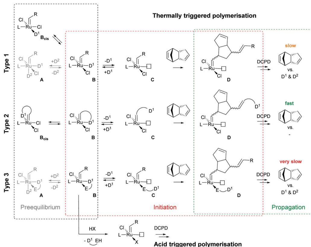
**Scheme 1** Most common avenues towards latent Ru-based initiators. L is typically a phosphine or an N-heterocyclic olefin; D<sup>1</sup> and D<sup>2</sup> are typically  $\sigma$ - or  $\pi$ -donor ligands such as amines, phosphines or N-heterocyclic carbenes; E is typically O or S; and R is typically an organic rest like a phenyl group.
