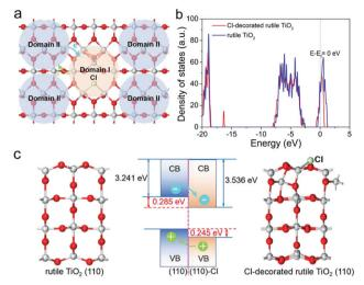
Fig. 1 (a) Scheme of the surface domain heterojunction (SDH), (b) total density of states (TDOSs) of the rutile TiO<sub>2</sub>(110) face with and without Cl decoration, and (c) atomic structures and the band diagram of SDH.
