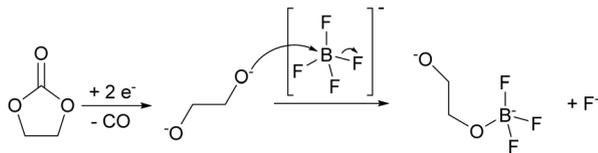
Fig. 7 Proposed mechanism for the anion decomposition upon reduction in  $\text{Ca}(\text{BF}_4)_2/\text{EC}:\text{PC}$  electrolytes. Further substitution of F by O can lead to cross-linked boron polymers.
