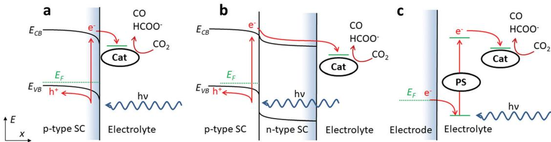
**Scheme 5** Possible photoelectrode configurations including molecular catalysts. (a) Catalyst at a p-type photocathode, (b) catalyst at a p-n photocathode, and (c) association between a catalyst and a sensitizer (PS) at a dark electrode surface.
