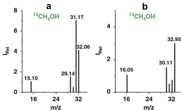
Fig. 15 GC/MS spectra and fragmentation pattern for the electrocatalyzed CO<sub>2</sub> conversion into CH<sub>3</sub>OH. Graphs show the mass fragmentation pattern of CH<sub>3</sub>OH (*m/z* 29 to 33) produced employing (a) <sup>12</sup>CO<sub>2</sub> or (b) <sup>13</sup>CO<sub>2</sub> as a reactant substrate. Reproduced with permission from ref. 250.
