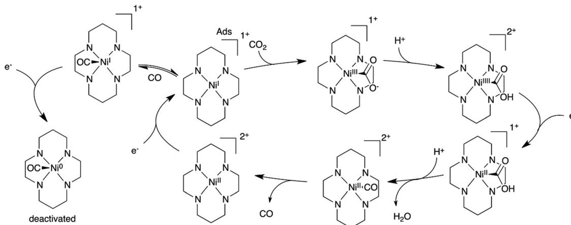
Scheme 1 Proposed electrochemical reduction mechanism of CO<sub>2</sub> to CO in water with the **Ni1** catalyst adsorbed at a Hg electrode.
