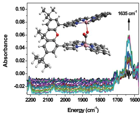
Fig. 14 Infrared spectro-electrochemistry data on a 1 mM solution of **Co<sub>2</sub>3** in  $\text{CH}_3\text{CN}$  (0.1 M  $n\text{-Bu}_4\text{NPF}_6$ , 0.5 M TEA) under  $\text{CO}_2$  at potentials between  $-0.35 \text{ V}$  and  $-0.85 \text{ V}$  vs. Ag pseudo-reference. Inset: Calculated structure of the  $\text{CO}_2$ -reduced complex adduct identified at  $1635 \text{ cm}^{-1}$ . Adapted with permission from ref. 40. Copyright 2019, Springer Nature.
