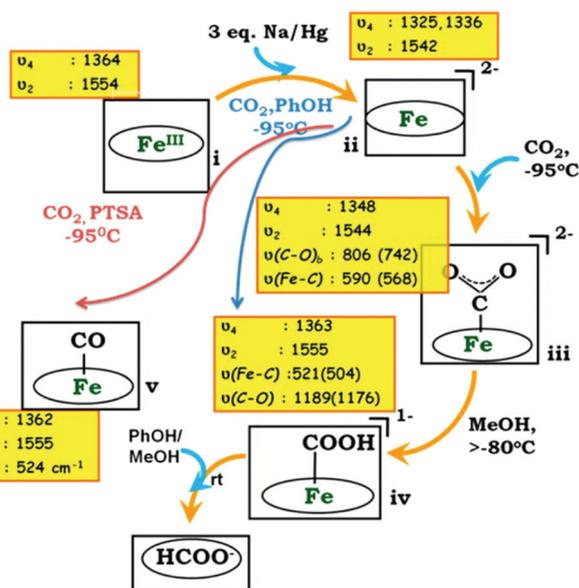
Fig. 7 Proposed mechanism for CO<sub>2</sub> reduction with **Fe20**, from Raman spectroscopic detection of intermediates. Reprinted with permission from ref. 38. Copyright (2015) American Chemical Society.
