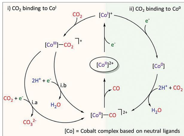
Fig. 8 Proposed mechanism of  $\text{CO}_2$  reduction with **Co27**. During CPE at the  $\text{Co}^{\text{II}}$  wave, trace amounts of CO were released. A formal oxidation state is given for the different Co species. Reprinted with permission from ref. 41. Copyright (2020) American Chemical Society.
