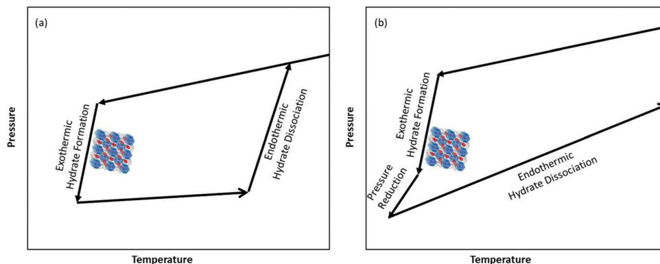
Fig. 27 Two modes of hydrate cold storage technology, namely heating (a) and (b) depressurising for cooling (based on Cheng *et al.*<sup>920</sup>).
