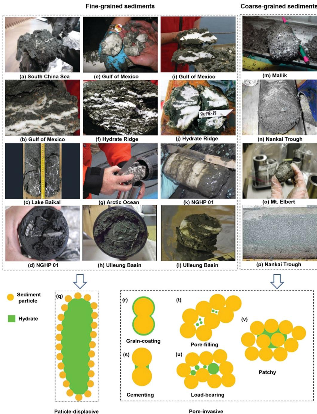
Fig. 8 Core-scale hydrate morphology in HBS samples and conceptual pore-scale habits for fine-grained and coarse-grained sediments (reprinted with permission from Ren *et al.*,<sup>403</sup> Copyright 2020 Elsevier Ltd).
