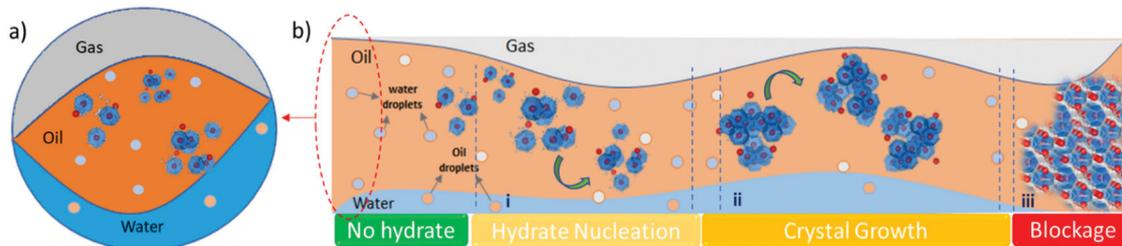
**Fig. 14** (a) Schematic model of multiphase flow in pipeline, where hydrate crystal aggregates could flow in gaseous, oleic, and aqueous phases, and/or could deposit onto the pipe solid surface; (b) schematic diagram of the drivers of hydrate crystals formation and aggregation in hydrocarbon transportation pipelines and three-step process of (i) hydrate nucleation, (ii) crystal growth, and (iii) blockage.
