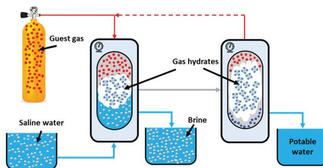
Fig. 28 Schematic diagram of the clathrate hydrate-based desalination process. Seawater is contacted with an appropriate hydrate former such as  $\text{CO}_2$  at desired thermodynamic conditions to form clathrate hydrates while excluding salts from the crystalline structure. The hydrate crystal can then be removed from the brine and dissociated to drinking water and hydrate former which could be recycled.
