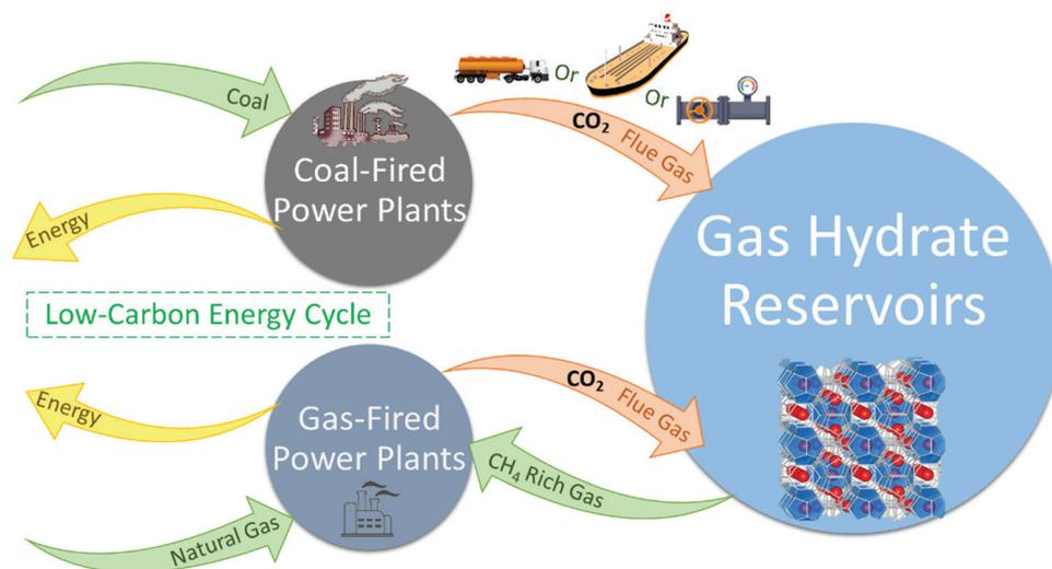
Fig. 24 Illustration of the principal mechanism of the direct injection of flue gas for methane recovery from gas hydrate reservoirs and CO<sub>2</sub> capture and storage simultaneously (adapted with permission from Hassanpouryouzband *et al.*,<sup>81</sup> Copyright 2019 Springer Nature).
