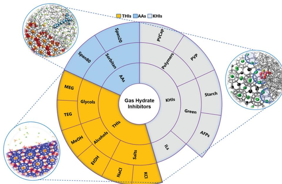
Fig. 15 Schematic examples of various types of gas hydrate inhibitors: THIs, KHIs, and AAs, and corresponding molecular interactions with clathrate hydrates.
