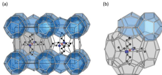
Fig. 4 (a) The structure of TBAB hydrate ((C<sub>4</sub>H<sub>9</sub>)<sub>4</sub>N<sup>+</sup>·Br<sup>-</sup>·38H<sub>2</sub>O). The solid lines represent the unit-cell of each hydrate. (b) Magnification of TBAB hydrate structure near tetra-*n*-butylammonium cation. The blue shaded dodecahedral cages are empty, and as such are candidates for engaging small molecules.
