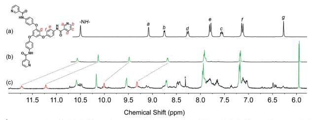
Fig. 2  $^{1}$ H NMR spectra for L (a), 1.12NO<sub>3</sub> (b), and after addition of 12 equiv. of NaC<sub>12</sub>H<sub>25</sub>OSO<sub>3</sub> into 1.12NO<sub>3</sub> (c) in Me<sub>2</sub>SO- $d_6$ . The 1.12NO<sub>3</sub> and 2.12C<sub>12</sub>H<sub>25</sub>OSO<sub>3</sub> resonances are indicated by the green and red signals, respectively
