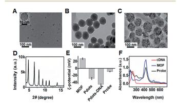
Fig. 4 TEM images of (A) P1 dots, (B) PCN-224 NPs, and (C) probe. (D) PXRD pattern of MOF nanoparticles. (E)  $\zeta$ -Potential characterization. (F) UV-vis absorbance of MOF NPs, cDNA, and the probe.
