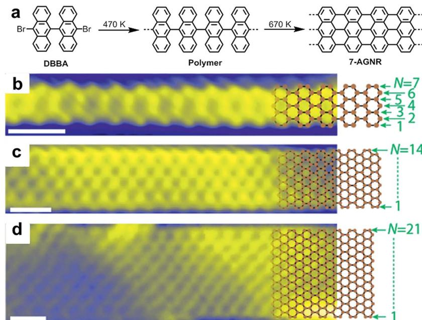
Fig. 2 Bottom-up synthesis of atomically precise AGNR from 10,10'-dibromo-9,9'-bianthryl (DBBA) monomer. (a) Synthetic route toward 7-AGNR. (b–d) STM images of 7-, 14-, and 21-AGNR with partially superimposed  $sp^2$  carbon framework structures. Reproduced with permission.<sup>97</sup> Copyright (2017) American Chemical Society.
