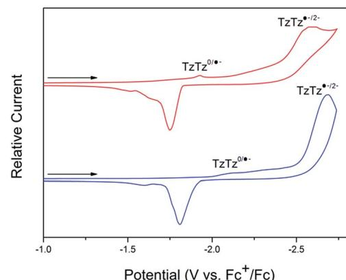
Fig. 2 Solid state CV of **1-Zn** (red) and **2-Cd** (blue) in the cathodic region, performed at a scan rate of 100 mV s<sup>−1</sup> in 0.1 M [*n*-Bu<sub>4</sub>N]PF<sub>6</sub>/MeCN.
