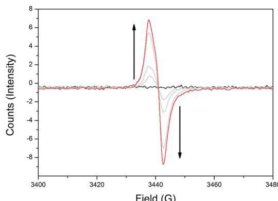
Fig. 3 Solid state EPR SEC of **1-Zn** in 0.1 M  $[n\text{-Bu}_4\text{N}] \text{PF}_6$ /MeCN, showing the appearance of the TzTz organic radical signal at  $g = 2.0043$  upon initial reduction.
