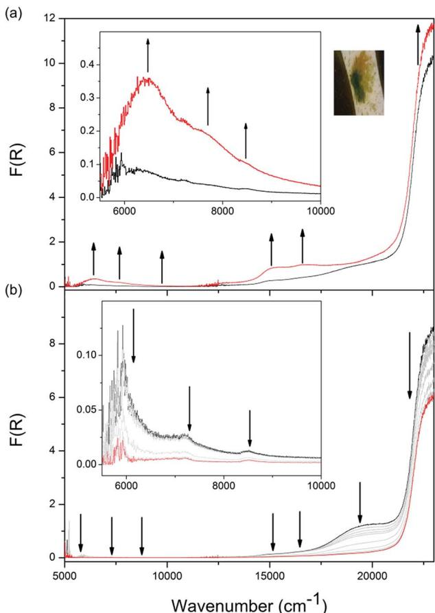
**Fig. 5** Solid state Vis-NIR SEC of **2-Cd** in 0.1 M [*n*-Bu<sub>4</sub>N]PF<sub>6</sub>/MeCN with arrows indicating progression of spectral bands at an applied potential of (a) −2.4 V with image of the green reduced frameworks provided; (b) −2.4 V after this potential was held for 40 min. Insets show the NIR regions for each plot.
