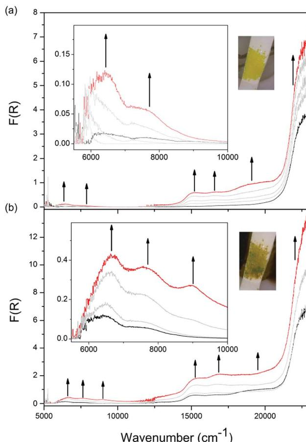
Fig. 4 Solid state Vis-NIR SEC of **1-Zn** in 0.1 M  $[n\text{-Bu}_4\text{N}] \text{PF}_6$ /MeCN with arrows indicating progression of spectral bands at an applied potential of (a)  $-2.1$  V; (b)  $-2.4$  V, with insets showing the NIR region as well as photos displaying the colour of the frameworks at respective potentials.
