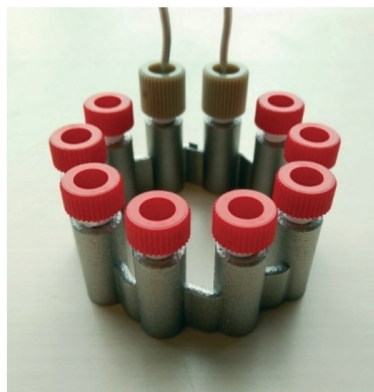
Fig. 6 3D printed CSTR cascade (AP01) closed with standard HPLC fittings. The 3D printed 10–32 UNF thread had to be refined after the printing.
