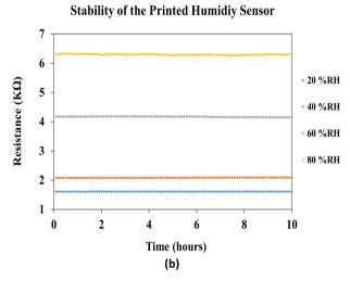
Fig. 16 (a) Transient response of the printed humidity sensor and (b) stability of the printed humidity sensor.
