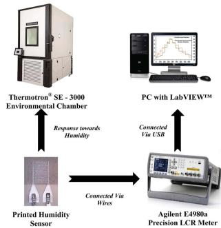
Fig. 7 Experimental setup.
