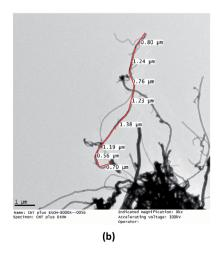
Fig. 8 TEM micrographs of MWCNTs showing (a) a diameter of  $\approx$  20–30 nm for the MWCNTs and a diameter of  $\approx$  80–90 nm for the MWCNT agglomerates, and (b) a length of  $\approx$  8–17  $\mu$ m for the MWCNTs.
