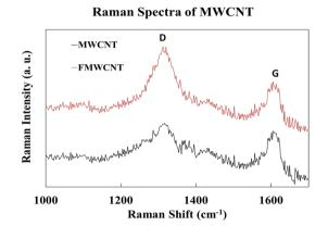
Fig. 10 Raman spectra of MWCNTs and FMWCNTs.
