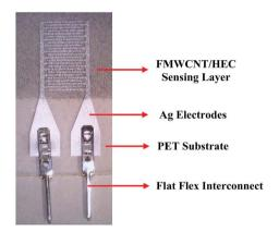
Fig. 5 Photograph of the printed sensor.
