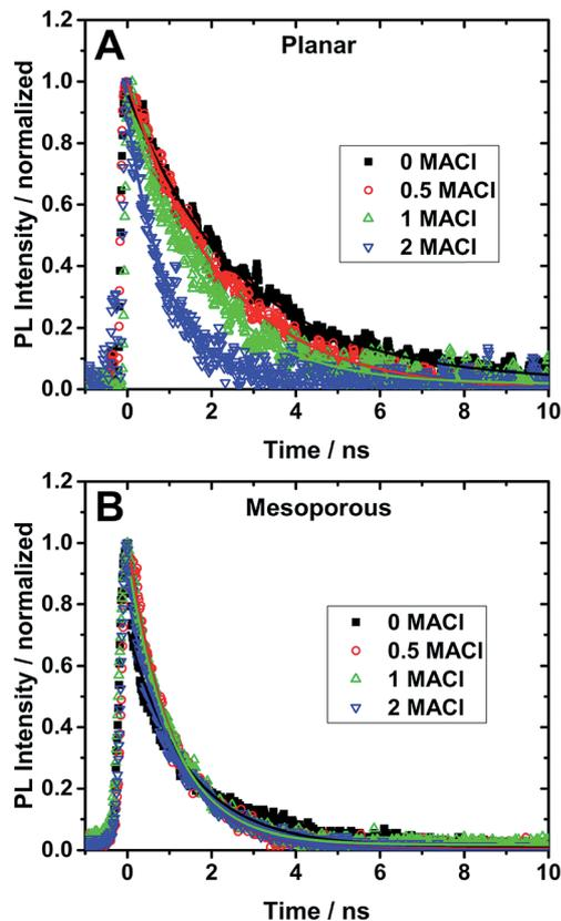
Fig. 4 TRPL decay dynamics (symbols) and their fits (lines) of perovskite films on (A) planar  $\text{TiO}_2$  and (B) mesoporous  $\text{TiO}_2$  coated FTO substrates excited using 480 nm light. The lifetimes obtained from the single exponential fits are reported in Table 1.
