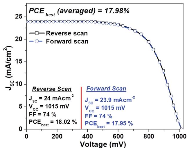
Fig. 5  $J$ - $V$  curves (both in the forward and reverse scans) for the best-performing device with MAPbI<sub>3</sub> micro-needles.
