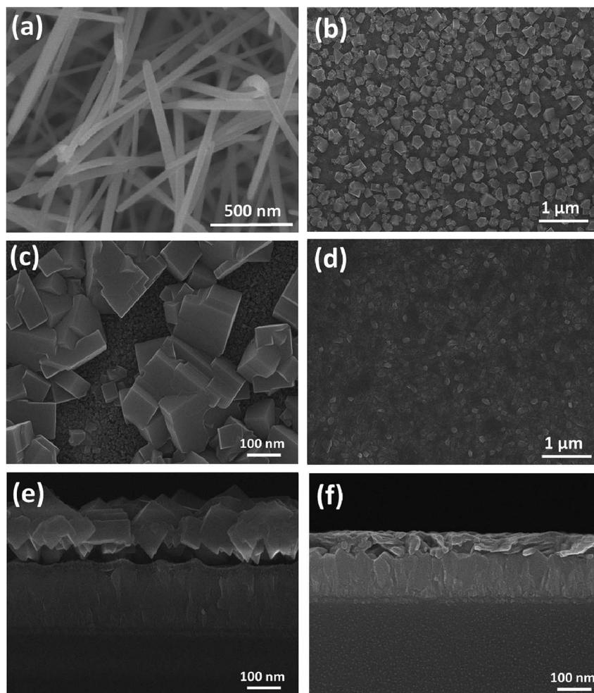
Fig. 2 Plane-view SEM micrographs showing (a) a magnified view of PbI<sub>2</sub> micro-needles and (b) nano-cubes of the perovskite, (c) a magnified view of perovskite nano-cubes and (d) MAPbI<sub>3</sub> micro-needles, and cross-sectional SEM images of FTO glass substrate/ZnO compact layer/(e) perovskite nano-cubes and (f) MAPbI<sub>3</sub> micro-needles, respectively.
