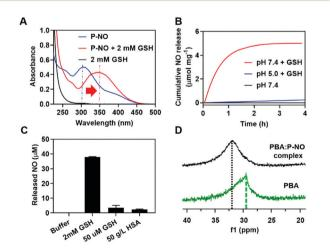
Fig. 1 Characteristics of P-NO. (A) UV-Vis spectra of P-NO with or without GSH. (B) GSH- and pH-dependent NO release. (C) HSA-independent NO release at pH 7.4. (D) <sup>11</sup>B-NMR of the PBA:P-NO mixture
