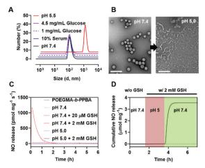
Fig. 2 Characteristics of P-NO-PMs. (A) Size distribution of P-NO-PMs dependent on different physiological conditions. (B) TEM image of P-NO-PMs at pH 7.4 and pH 5.0. Scale bar is 100 µm. (C) NO release profiles of P-NO-PMs under various physiological conditions. (D) NO release profile of P-NO-PMs under physiological buffer (white box), endolysosomal (pH 5, 2 mM GSH; red box) and, cytosolic conditions (pH 7.4, 2 mM GSH; areen box)
