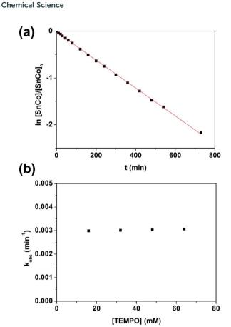
Fig. 8 (a) First-order kinetic plot on 1 with 10 equivalents of TEMPO, and (b) zeroth-order kinetic plot on TEMPO. Conditions: 1.6 mmol L $^{-1}$  of 1, C $_6$ D $_6$ , 70.0 °C, in the dark and under a N $_2$  atmosphere.
