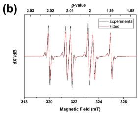
Fig. 7 Spin trapping of 2. (a) EPR monitoring of a toluene solution of 1 and PBN at  $-50\,^{\circ}$ C, under visible light irradiation (Xe lamp, 420–780 nm), and (b) fitting of the EPR spectrum of the same sample, recorded at  $-20\,^{\circ}$ C.
