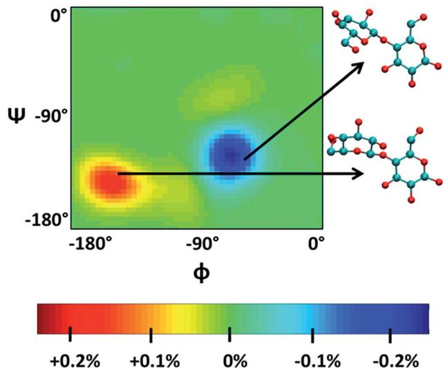
Fig. 9  $\phi$ - $\psi$  difference maps ([Bmim][Cl]-water) for the most populated basin O ( $-180^\circ < \phi/\psi < 0^\circ$ ) at 375 K and 450 K. The two examples of cellobiose structures characterize the difference between structures from the "Bmim" basin (red) and those from the "water basin" (blue).<sup>93</sup> Reproduced from ref. 93 with permission from the American Chemical Society.
