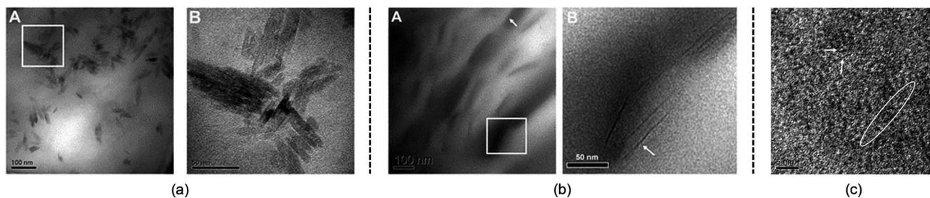
Fig. 11 TEM photographs of microcrystalline cellulose at different scales treated by [Amim][Cl] after 1 h. (a) is 100 nm, (b) is 50 nm, (c) is 5 nm (room temperature for 4 months).<sup>111</sup> Reproduced from ref. 111 with permission from the Royal Society of Chemistry.
