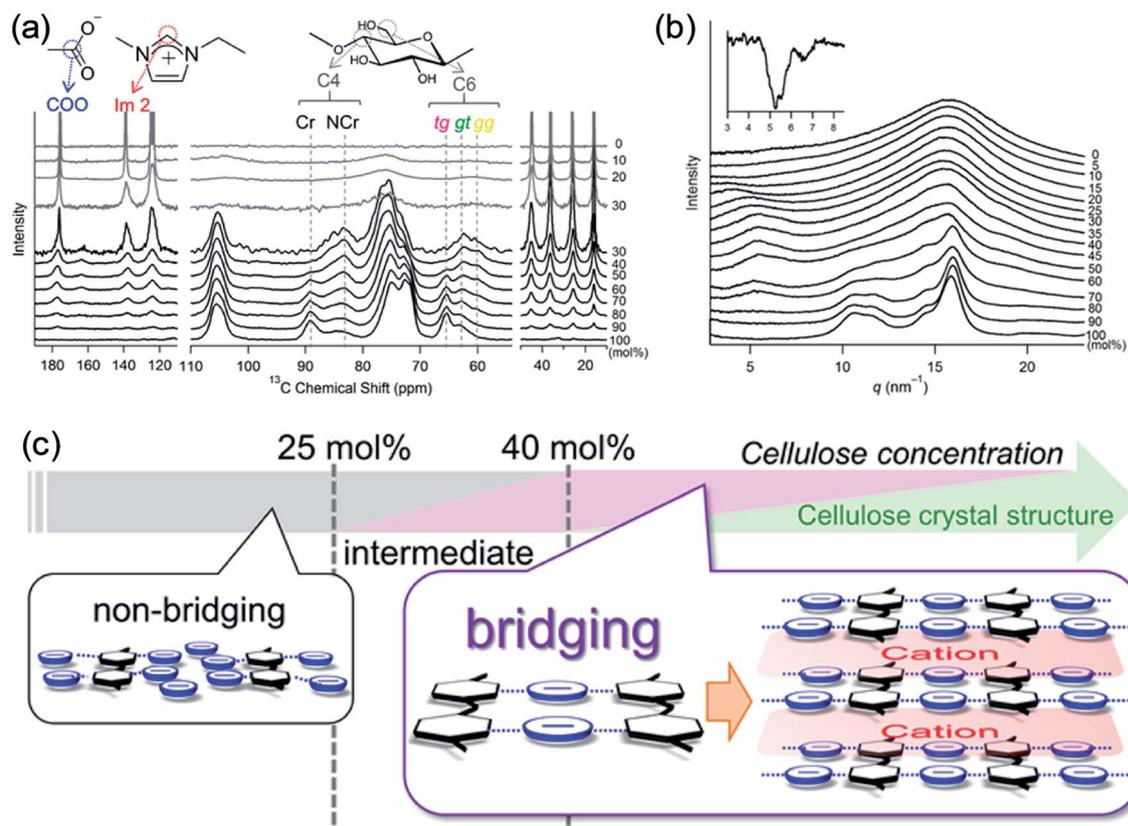
Fig. 5 (a)  $^{13}\text{C}$  solid-state NMR spectra obtained at 5 kHz of MAS for the cellulose/[Emim][OAc] mixtures. (b) WAXS patterns of cellulose/[Emim][OAc] mixtures. (c) Schematic summary of non-bridging to bridging state transformation with the increase of cellulose concentration in [Emim][OAc].<sup>50</sup> Reproduced from ref. 50 with permission from the American Chemical Society.
