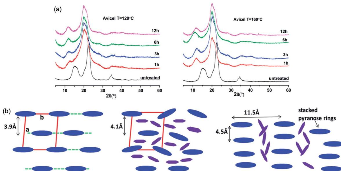
Fig. 6 (a) XRD patterns of Avicel cellulose in [Emim][OAc] at 120 °C (left) and 160 °C (right).<sup>55</sup> (b) Schematic representation of the arrangement of cellulose crystalline structure (blue) and the intercalated ILs (purple).<sup>56</sup> Reproduced from ref. 55 and 56 with permission from the American Chemical Society.
