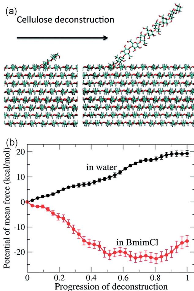
Fig. 16 (a) The peeling process of cellulose by means of steered molecular simulation. (b) The potential mean force (PMF) of the peeling process in water and ionic liquids.<sup>99</sup> Reproduced from ref. 99 with permission from the American Chemical Society.
