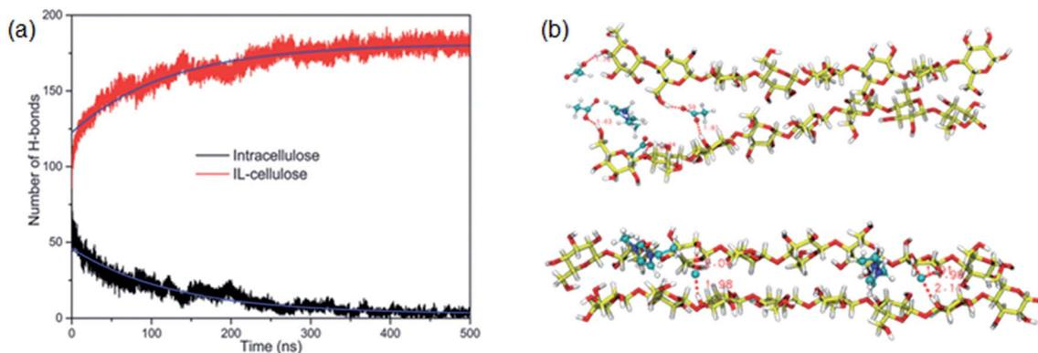
Fig. 13 (a) The change of intracellulose and cellulose–IL H-bonds during the simulation of a cellulose bunch in [Emim][OAc]. (b) Snapshots of H-bond formation between cellulose chains and ILs.<sup>105</sup> Reproduced from ref. 105 with permission from the PCCP Owner Societies.
