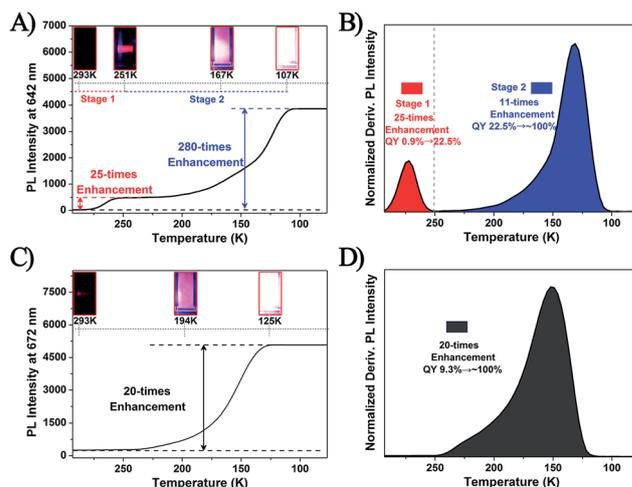
Fig. 6 The PL intensity at the fixed points of (A) 642 nm for the  $\text{Ag}_{29}(\text{BDT})_{12}(\text{TPP})_4$  NC and (C) 672 nm for the  $\text{Pt}_1\text{Ag}_{28}(\text{S-Adm})_{18}(\text{TPP})_4$  NC at different temperatures. Insets: the digital photographs of each NC in DMF solution under UV light. The derivative results for PL intensity of (B)  $\text{Ag}_{29}(\text{BDT})_{12}(\text{TPP})_4$  and (D)  $\text{Pt}_1\text{Ag}_{28}(\text{S-Adm})_{18}(\text{TPP})_4$  NCs.
