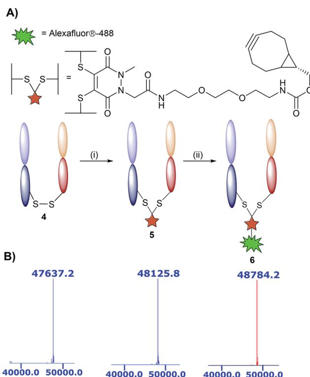
**Fig. 2** Modification of TRAZ F(ab) with strained alkyne functionalised pyridazinedione **3**. (A) Scheme 2: reagents and conditions: (i) **3**, TCEP·HCl, BBS pH = 8.0 (2 mM EDTA), 4 °C, 15 h; (ii) Alexafluor-488-N<sub>3</sub> BBS pH = 8.0 (2 mM EDTA). (B) LCMS data showing native **4**, conjugated **5**, and clicked TRAZ F(ab) **6**. Spectra have been annotated for clarity, see Fig. S7, S9 and S12 in the ESI† for full spectral data.
