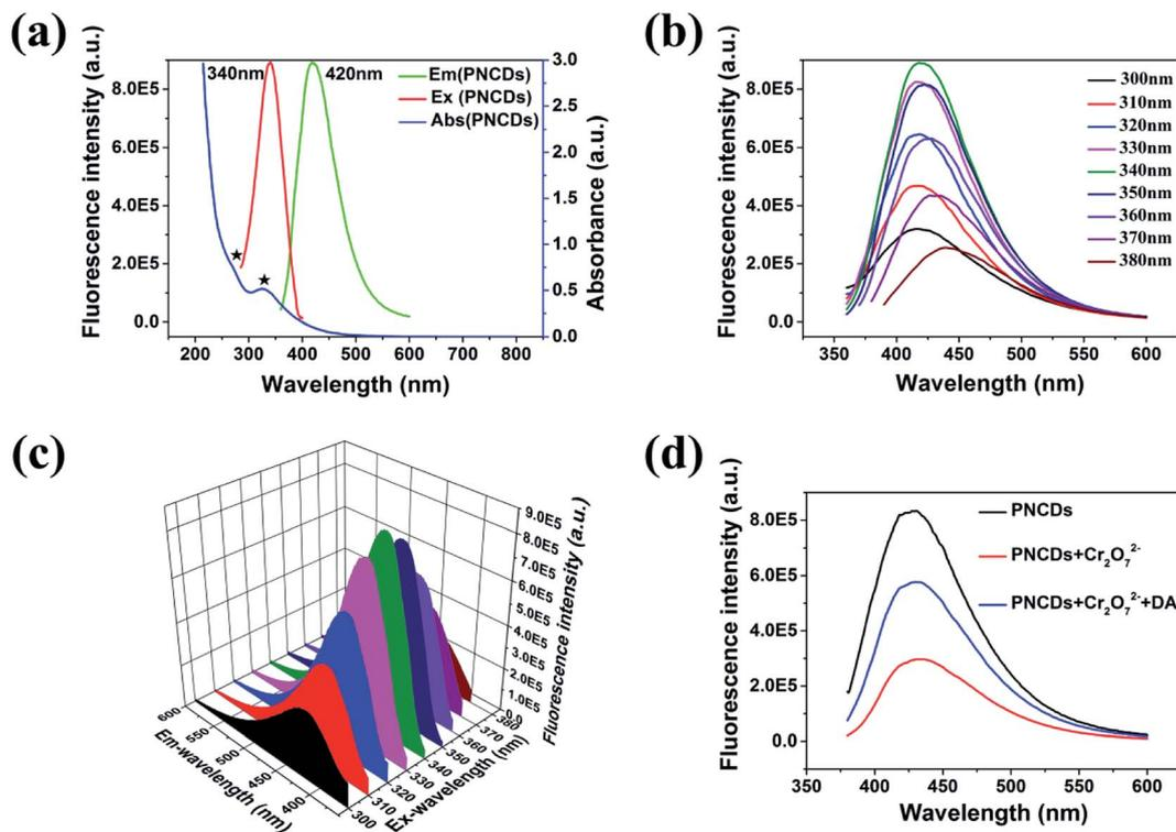
Fig. 3 (a) UV-vis absorption (blue line), PL excitation (red line), and emission (green line) spectra of PNCDs in aqueous solution ( $0.30 \text{ mg mL}^{-1}$ ). (b) Excitation-dependent PL behavior of PNCDs. (c) 3D wall spectra of the PNCDs with different excitation wavelength. (d) Fluorescence emission spectra of PNCDs at different conditions: PNCDs (black line), PNCDs +  $\text{Cr}_2\text{O}_7^{2-}$  (red line), PNCDs +  $\text{Cr}_2\text{O}_7^{2-}$  + DA (blue line).
