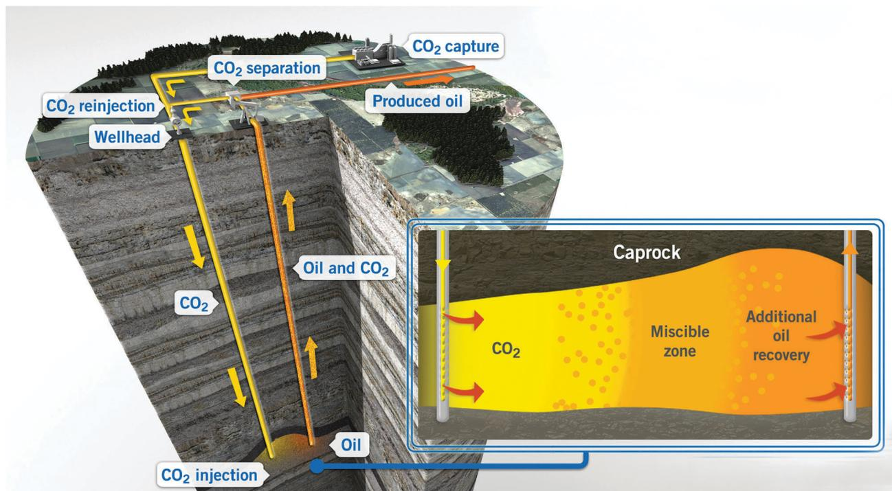
Fig. 19 Schematic diagram of CO<sub>2</sub>-EOR process. Source: Global CCS Institute.<sup>964</sup>
