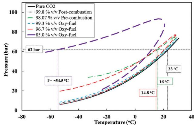
Fig. 17 Boundaries of VLE region in pressure–temperature phase diagram for pure CO<sub>2</sub>, pre-combustion, post-combustion and oxy-fuel streams (85 and 96.7% v/v CO<sub>2</sub>) calculated using PR EoS.<sup>808</sup>
