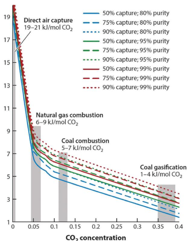
Fig. 27 Minimum work required for CO<sub>2</sub> capture based upon initial CO<sub>2</sub> concentration, capture rate, and final CO<sub>2</sub> purity.<sup>308</sup>
