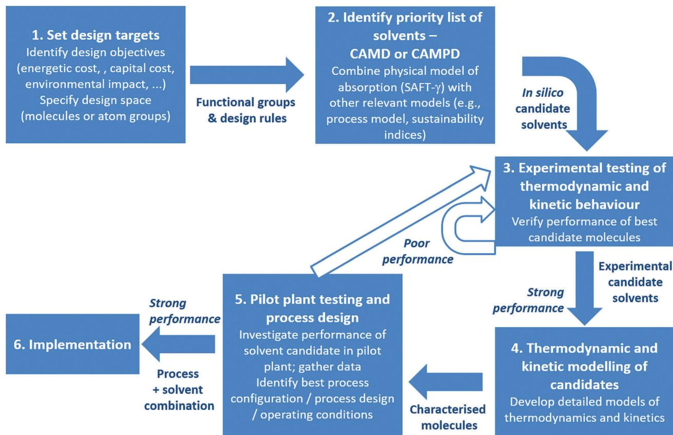
Fig. 16 An overview of an approach to the design of solvents and processes for CO<sub>2</sub> capture, highlighting the role of different modelling and experimental activities.
