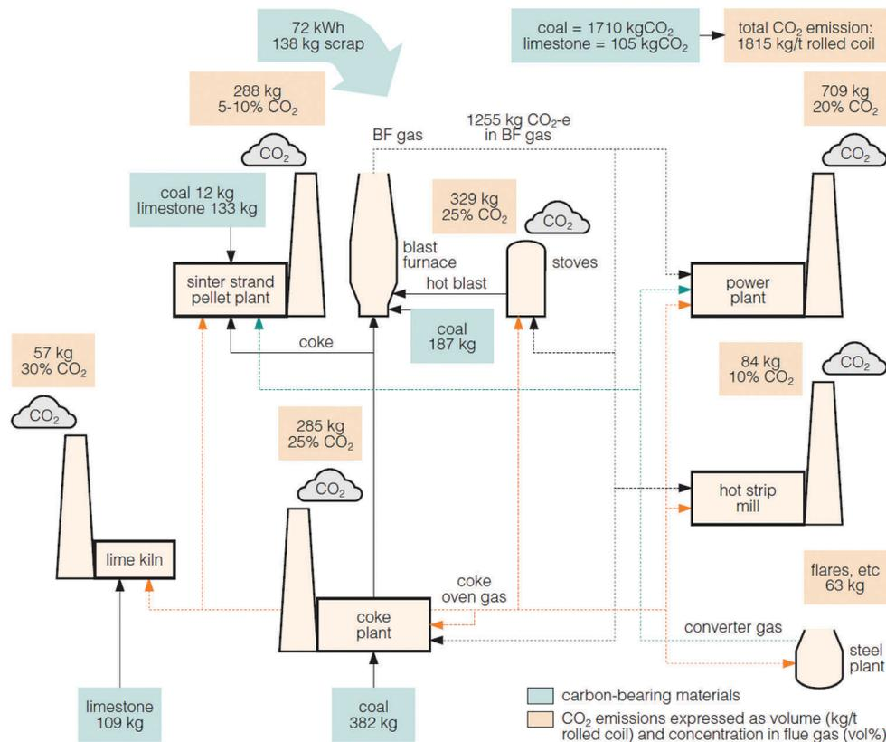
Fig. 8 A typical steel mill and the CO<sub>2</sub> emissions, which vary in concentration.<sup>117,118</sup>
