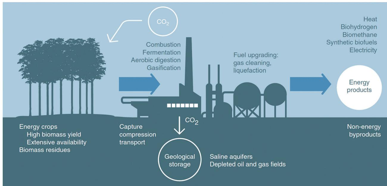
Fig. 23 Concept of bioenergy with carbon capture and storage (BECCS), courtesy of Nature.<sup>1065</sup>
