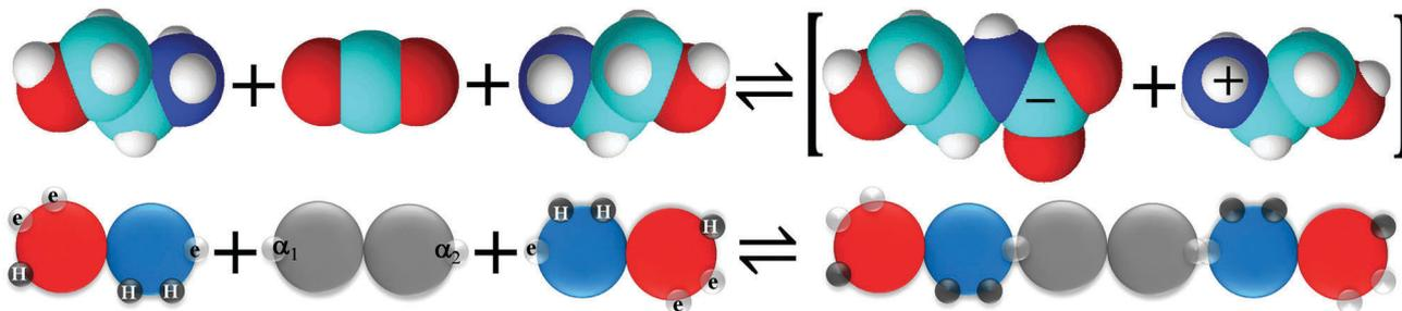
Fig. 13 SAFT physical model of  $\text{CO}_2$  chemisorption in aqueous MEA solution: the amine groups are depicted in dark blue, the hydroxyl groups in red, and  $\text{CO}_2$  in grey; the sites labelled "e" are the hydrogen-bond acceptor electron-lone pairs of the electronegative atoms, the sites labelled "H" are the donor hydrogen sites, and the sites labelled "a" are the sites mediating the reactions with  $\text{CO}_2$ .
