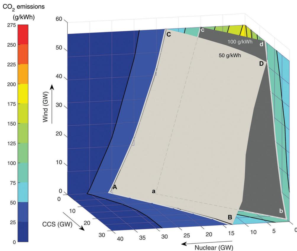
Fig. 5 The CO<sub>2</sub> emissions as a function of nuclear, CCS and wind build. The surfaces show the technology deployment requirements in order to meet the CCC targets for CO<sub>2</sub> emissions of 100 g kWh<sup>-1</sup> and 50 g kWh<sup>-1</sup>.
