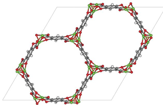
Fig. 9 Example of a MOF. Here the structure of Mg-MOF-74 is shown. This MOF exhibits the highest reported CO<sub>2</sub> uptake for unfunctionalised adsorbents.
