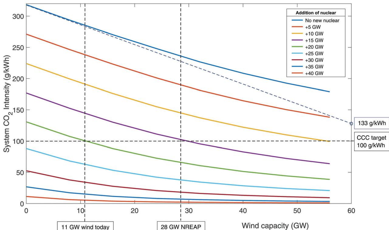
Fig. 4 The CO<sub>2</sub> emissions in 2030 as a function of wind and nuclear build when unabated CCGT is used as flexible back-up.
