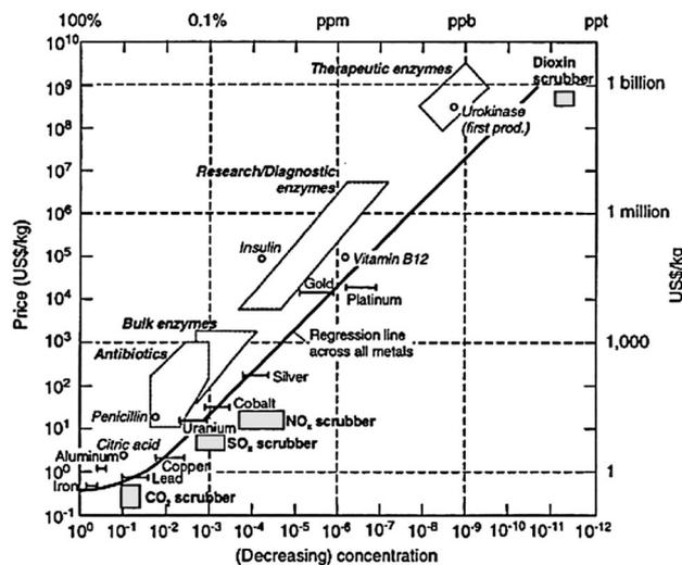
Fig. 28 Sherwood plot exhibiting the relationship between the concentration of a target material in a feed stream versus the cost of its removal.<sup>67</sup>
