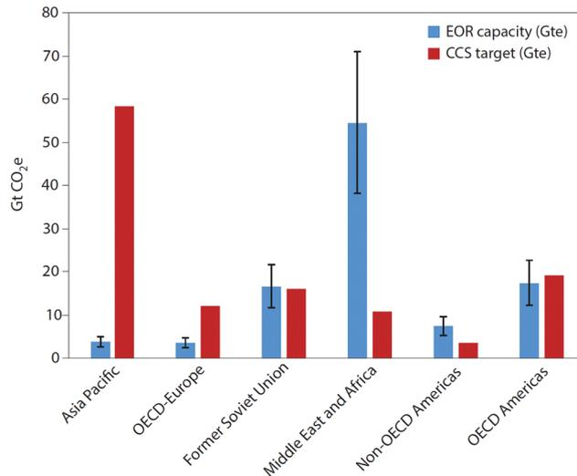
Fig. 20 Global CO<sub>2</sub>-EOR capacity compared with CO<sub>2</sub> mitigation targets. Figure reproduced from Mac Dowell *et al.*<sup>967</sup> Data from Dooley *et al.*,<sup>974</sup> IEA,<sup>975</sup> and CIA.<sup>976</sup> The error bars indicate an average calculated variance of 30%. The actual reported variance is in the range of 25–35%.
