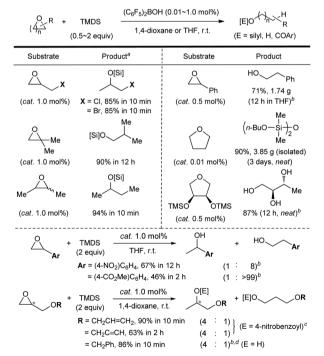
**Scheme 5** Substrate scope of the Piers' borane-catalysed hydrosilylation. <sup>a</sup> Yields were determined using <sup>1</sup>H NMR. <sup>b</sup> The desired alcohol products were isolated upon hydrolysis with saturated  $K_2CO_3$  in MeOH. <sup>c</sup> The crude products were *O*-benzoylated *in situ* through the reaction with 4-nitrobenzoyl chloride. <sup>d</sup> (*S*)-1-(Benzyloxy)propan-2-ol was obtained as a major product with >98% ee.
