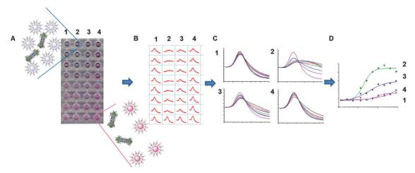
Fig. 1 Overview of the approach used to allow direct measurement of carbohydrate-lectin interactions by monitoring a colourimetric change (red to blue) due to aggregation of glycoAuNPs bound to lectins (A) and the use of absorbance spectra (B and C) in the formation of binding curves (D).
